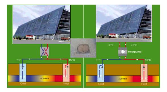
So in fact there will be a thermal balance and the water flow balance in the ATES. The capacity of the Aquifer Thermal Energy Storage is approx. 200 m $^3$ /h which corresponds with approx. 1.000 kW cooling energy at a temperature range of: 13  $^{\circ}$ C - 18  $^{\circ}$ C.
